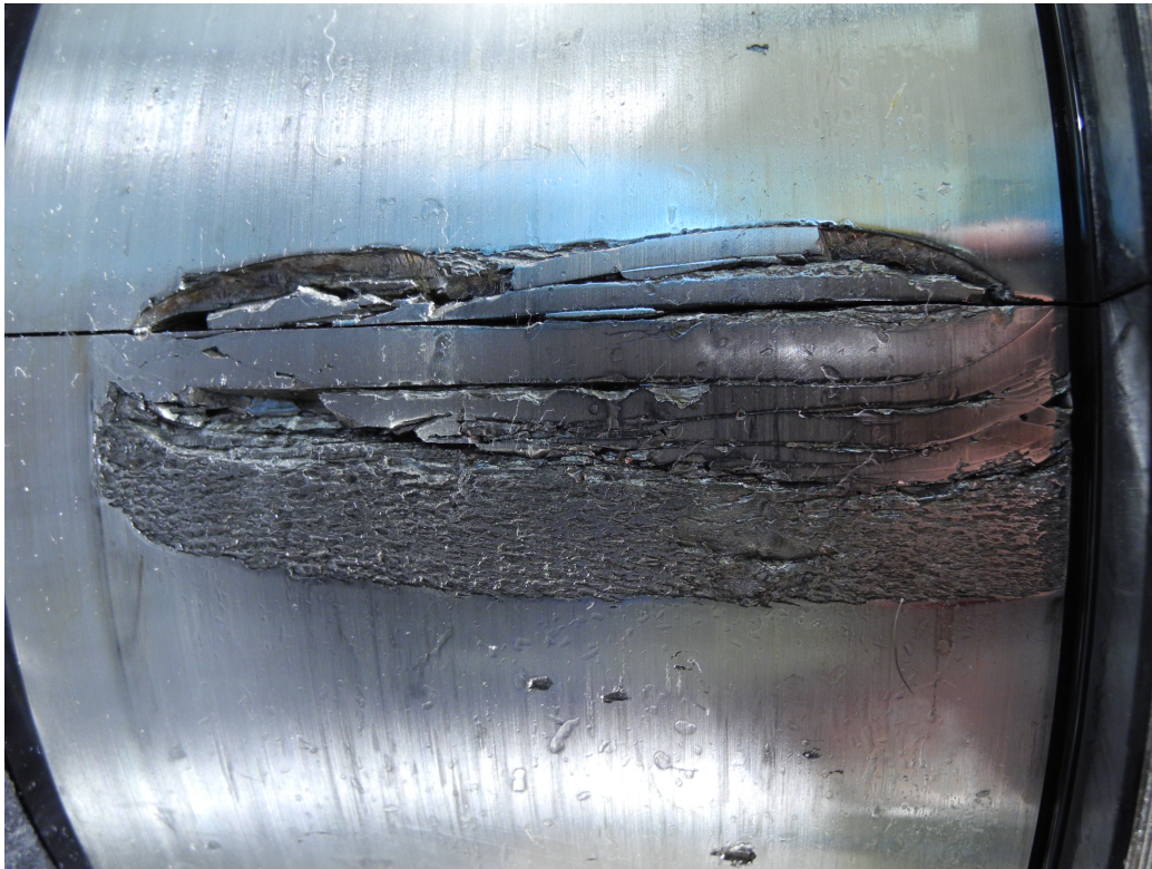
Figure 3: Failed wind turbine gearbox bearing (inner raceway, high speed shaft)
