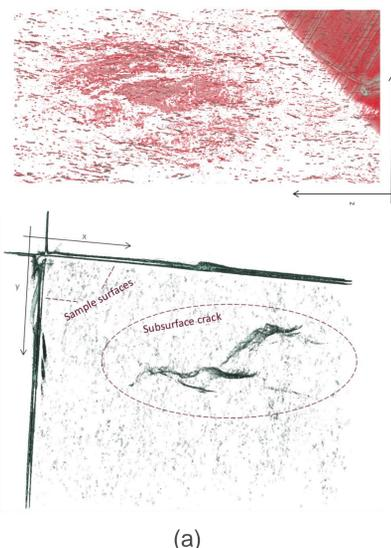
a) 3D reconstruction crack images from X-ray microtomography, b) WEC found in wind turbine bearing sample, c) WEC found in micro-pitting rig roller sample
